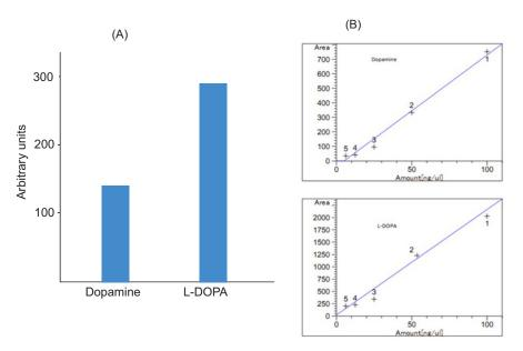
**Figure 3**. Figure 3A shows a typical signal obtained from the analysis of a standard and solution of commercial L-DOPA and dopamine using the proposed method. Data are the average results of three independent experiments. Figure 3B shows the regression equation and correlation coefficient (r) for L-DOPA and dopamine. The HPLC-based assays show a good level of linearity.
