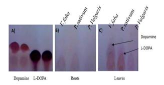
**Figure 2.** TLC analysis of L-DOPA and dopamine. A. Standard spots of catecholamines. B and C). The amount of L-DOPA and dopamine in roots and leaves of plant samples.
